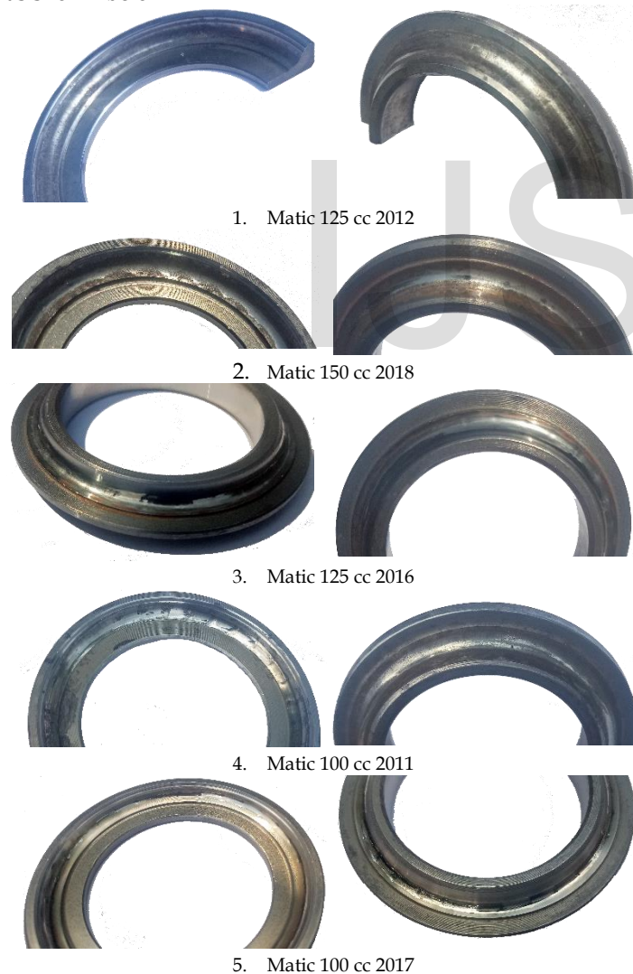
Fig. 4. Failed Steering Bearing several motorcycles.
